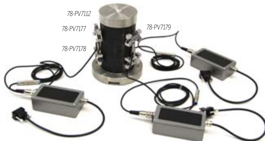
AMPT, Dynamic modulus, Uniaxial test set, including set of three LVDT transducers and mounting clamps.
