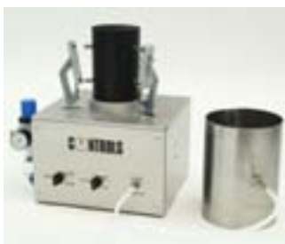
AMPT, Dynamic modulus, Uniaxial test set, detail of fitting system for gauge points and vacuum
