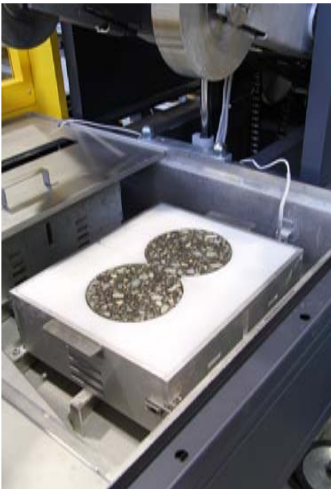
Mould adaptor for double 150 mm dia. Cylindrical samples to AASHTO T324
