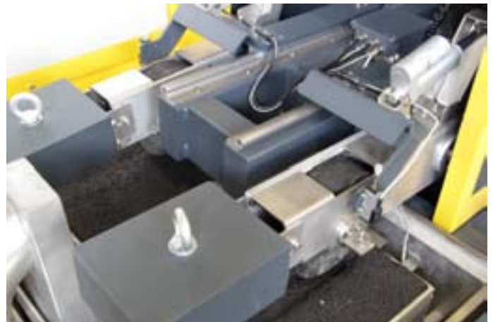
77-PV3UP10 Upgrading option. One of the two wheels is automatically lifted after test is completed continuing the test with the other wheel up to the rut target.
