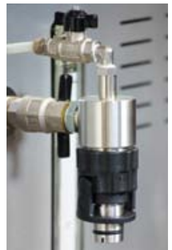
Detail of fast connection for Rotary evaporator flask, for bitumen solution sampling
