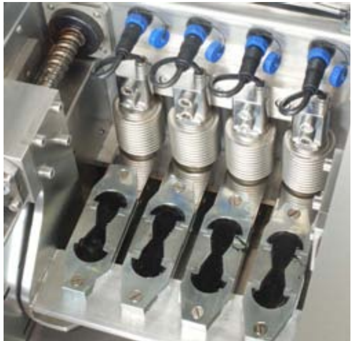
Detail of 81-PV10B02 and PV10C02 with four 81-PV10020 load cells and briquette moulds
