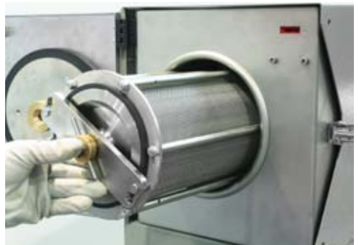
Placing the washing drum into the machine
